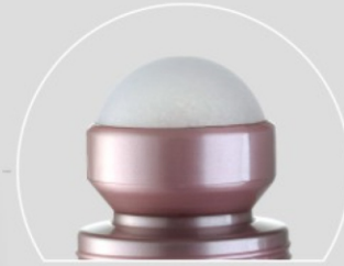
P3002 Volume:50ml Ball Diameter:35.56mm Height:93.7mm Material Cap:PET Bottle:PET Ball:PP
